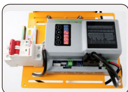
PWM variable frequency servo controller board
