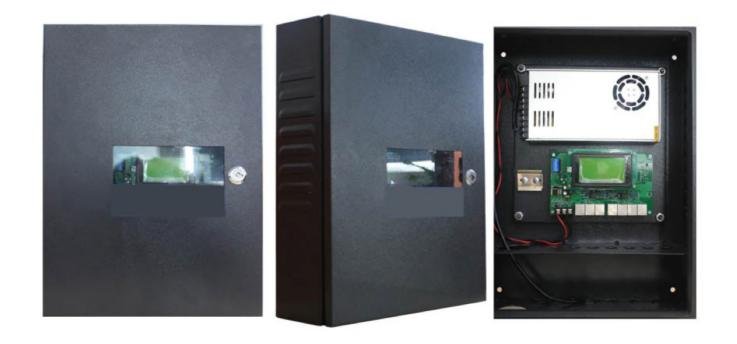
Data Collector works as a bridge which connects Centre Processor to Ultrasonic Sensors. It collects and transfers sensor information to Centre Processor for final processing, and also transfers availability information from Centre Processor to LED Displays. A Data Collector manages up to 60 unit Ultrasonic Sensors and 20 unit LED displays
