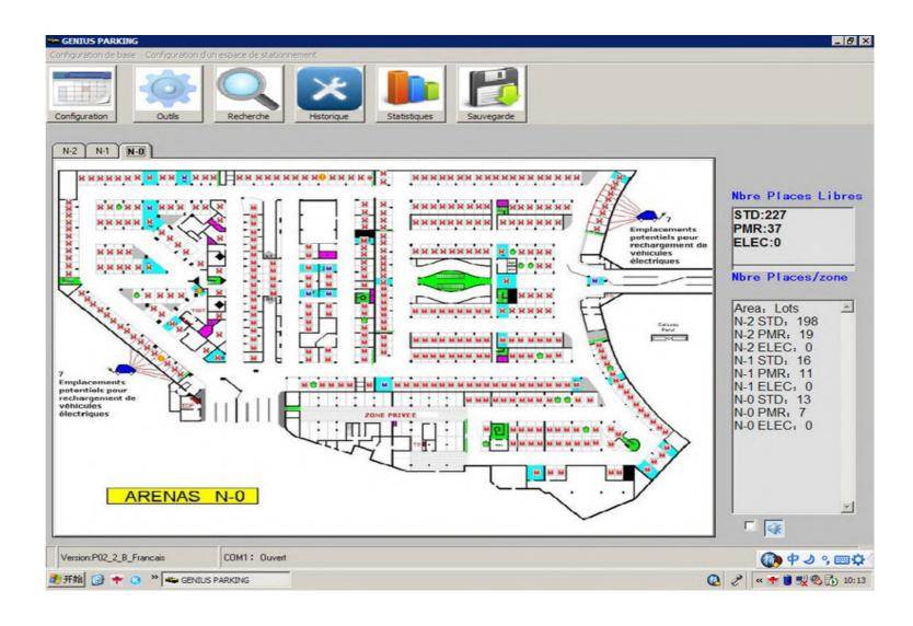
Multi-language, graphical application developed based on Window 7 OS & SQL database to display the occupancy status of parking spaces in real-time basis and provide various statistic reports for the management.
