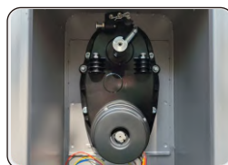
300W DC Servo Motor Alloy steel helical gear
